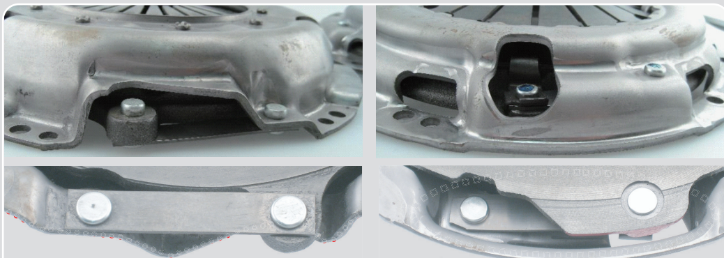
Straps and Levers are enclosed, increasing the cover rigidity.
